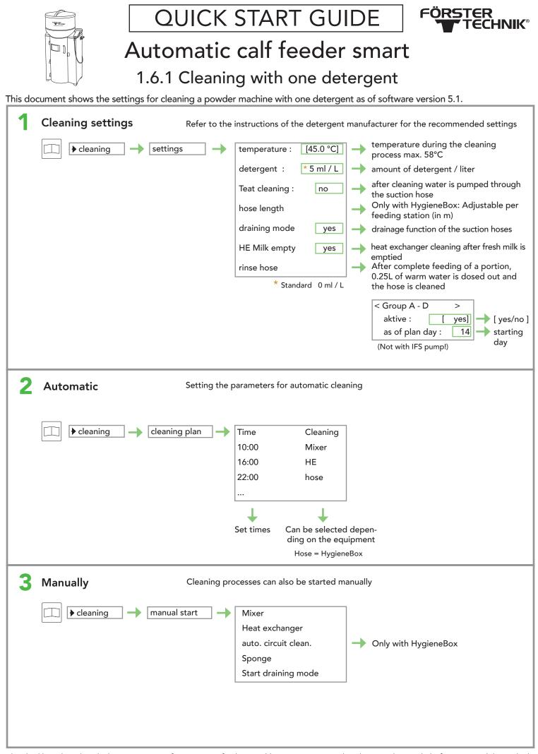
This checklist is based on the basic equipment of an automatic feeder. Possible extensions are not listed separately. Detailed information and the applicable warnings and safety instructions can be found in the corresponding operating instructions. (Status 23/09)
