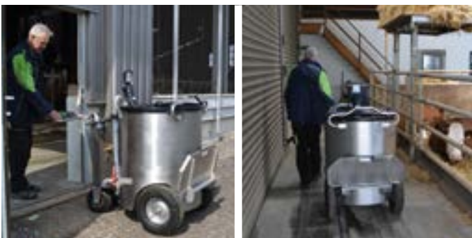
The four wheels and the electric drive ensure optimum driving stability - no matter where.
