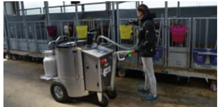
The desired feed amount is dosed precisely at the push of a button.
