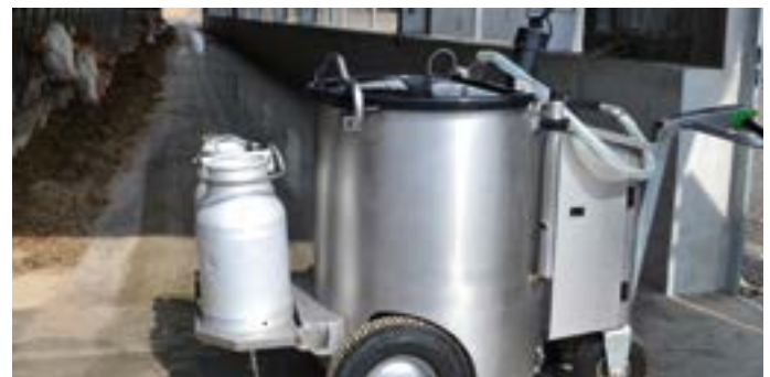
The optional foldable holder simplifies the transport of multiple milk jugs or buckets.
