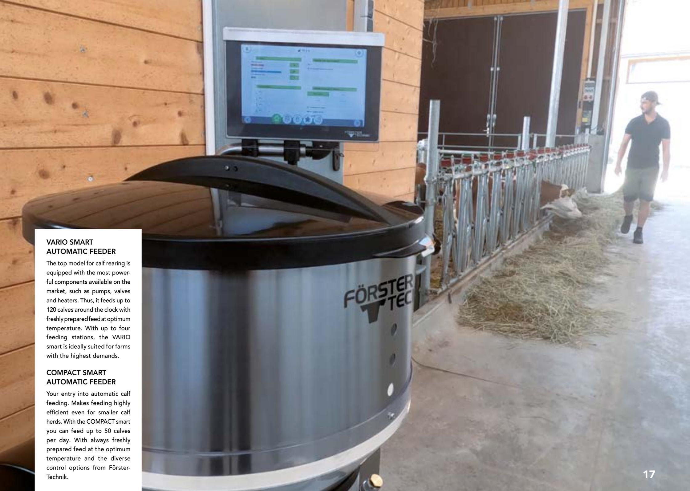
A large stainless steel automatic feeder is mounted on a wooden wall in a barn. The feeder has a black lid and a control panel with a touchscreen display showing a software interface. The brand name 'FÖRSTER TECH' is visible on the side of the feeder. In the background, a man in a dark shirt and shorts is walking through a long metal feeding station filled with hay.
