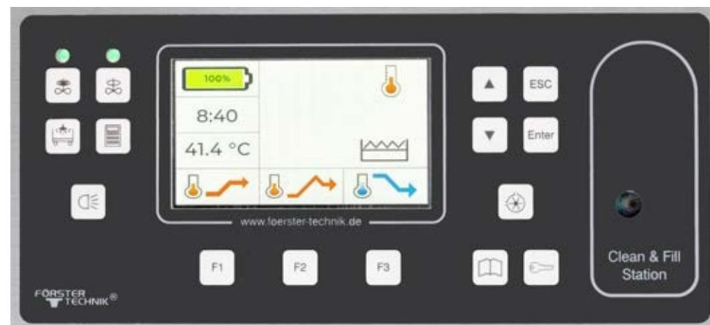
Fig. 3: LED color display with light-up keypad.
